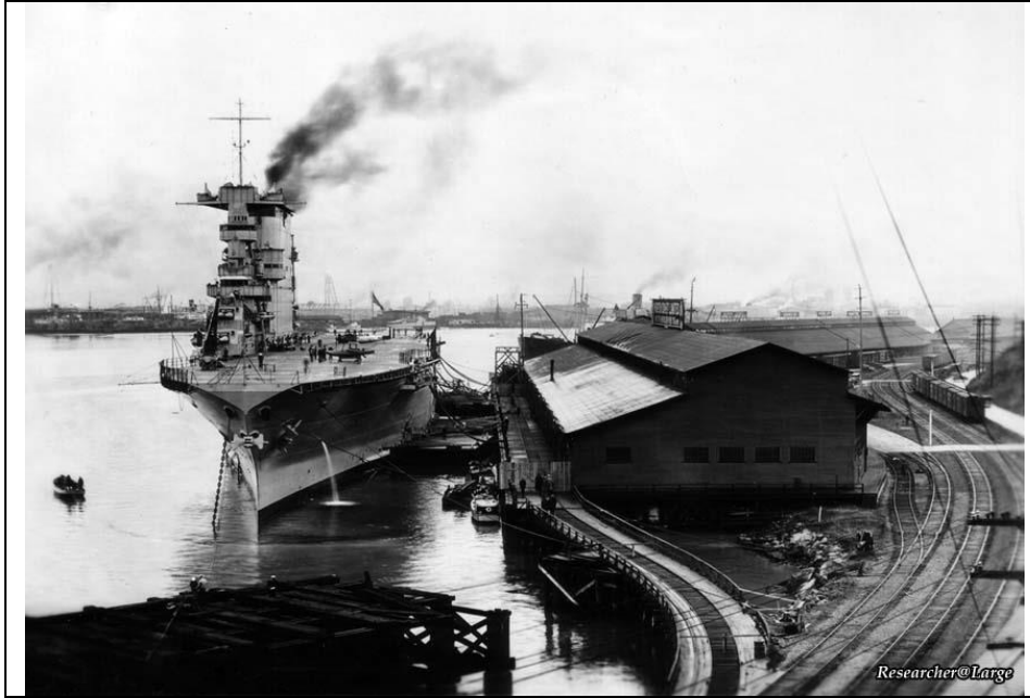
Figure EE-1 The Carrier Lexington Providing Electricity to the City of Tacoma 12
